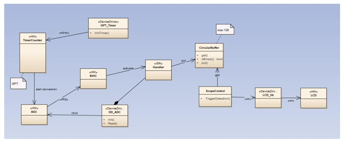
This is an example of a class diagram representing the components of a very simple digital scope. Stereotypes are used to document what type of thing is being represented by each class: HW, Device Driver, ISR, ...
