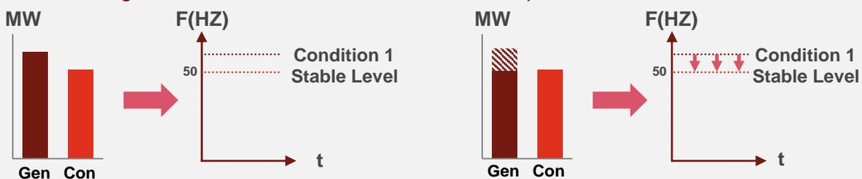
If the frequency falls below 50 HZ, consumption is higher than generation.
