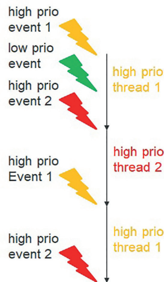
Fig. 64: Thread starvation of the low priority thread
