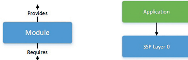
Fig. 47: Basic view of a module with interfaces (left) and application code using a module
