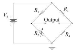
When the bridge is balanced, the output voltage is zero, and the products of resistances in the opposite diagonal arms are equal.
