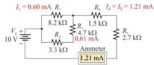
As a check on the currents, KVL can be applied to the outside loop. For this check, calculate  $V_1$ ,  $V_4$ , and  $V_5$ .
